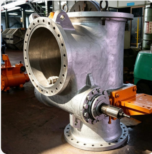
Main Stop Valve
